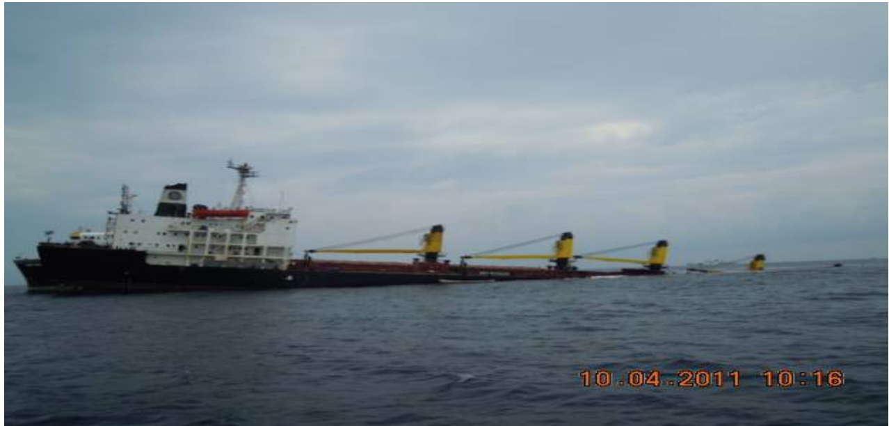
Photo no.24: 10 April, Side view with cargo hold no.1, 2 & 3 flooded
