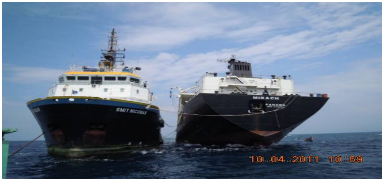
Photo no.26: “Smit Nicobar” salvage tug engaged in transfer of fuel from engine room
