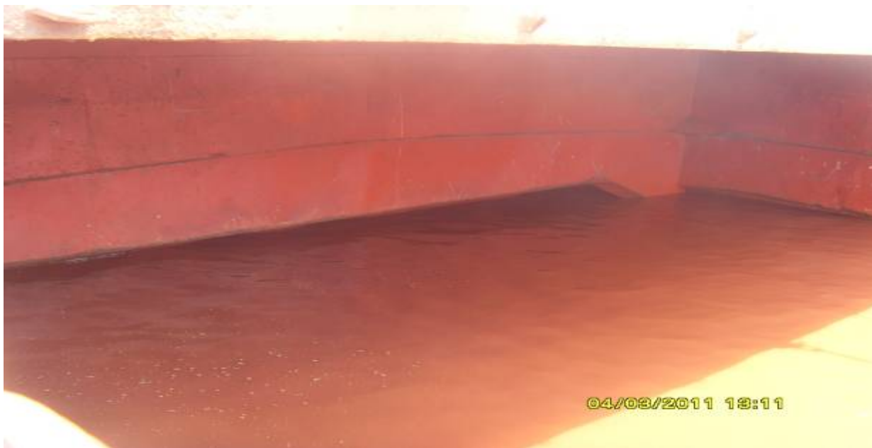
Photo no.8: 3 April 2011, flooded cargo hold no.1
