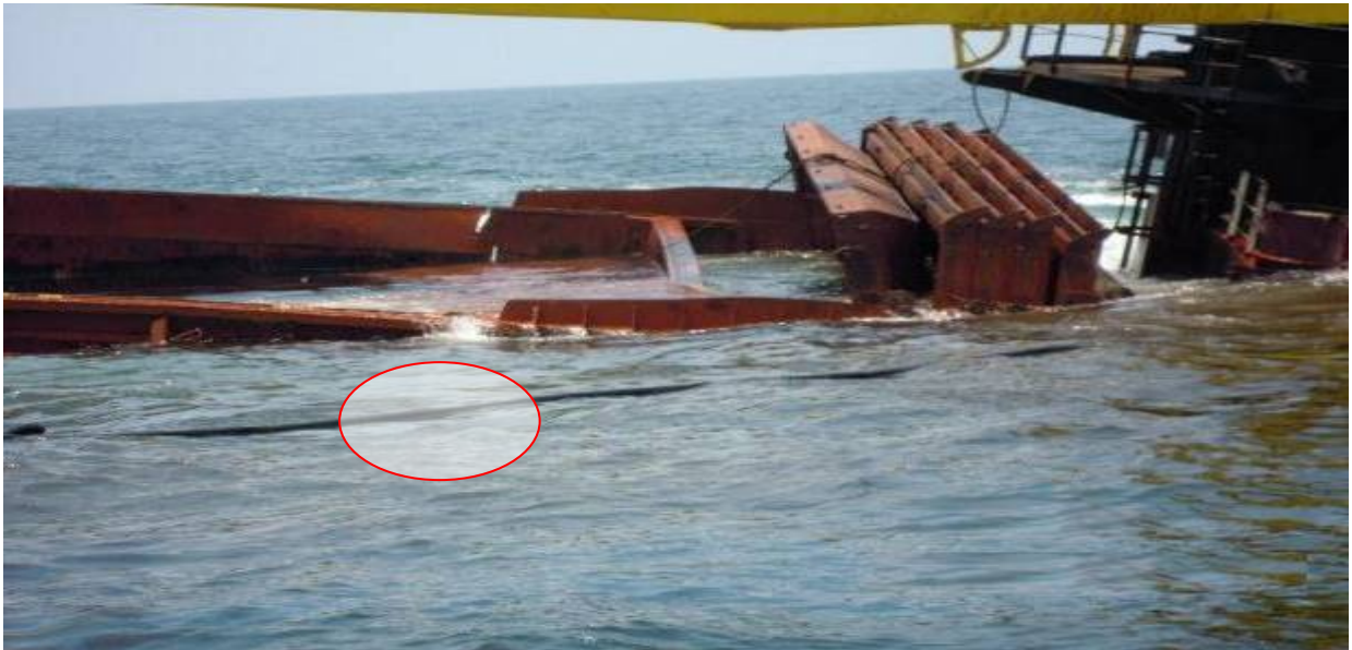
Photo no.22: 06 April, Cargo hold no.3 flooded, Crack on port side hatch coaming of no.3
