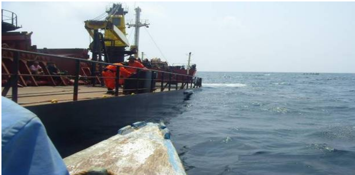
Photo no.13: 03 April, Salvage tug crew on board, vessel down by head
