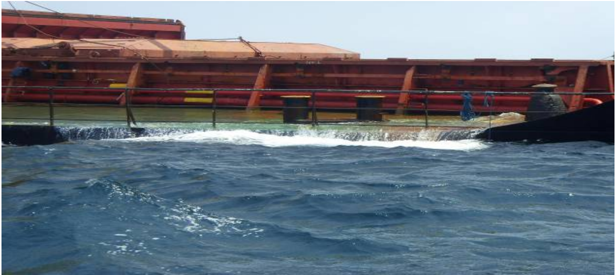
Photo no.12: 03 April, Sea water coming on starboard side forward main deck
